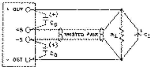
Figure 1- Output sense connections
